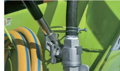
4.Spring loaded switch for water charging.
