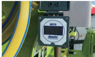
5.Digital water meter: Displays the amount of water added each time, and can be automatically reset.
