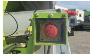
7.Emergence stop buttons: Four Emergence Stop buttons applied and covered by protections.
