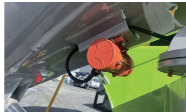
6.Vibrators: Vibrators mounted on the chute and the outlet to ensure the concrete dumping effectively.
